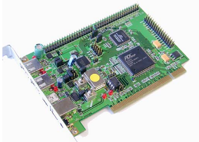
Figure 2-2: ISPI362 PCI Evaluation Board
